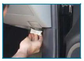
3. Insert one end of the "Y" cable back into the original slot
