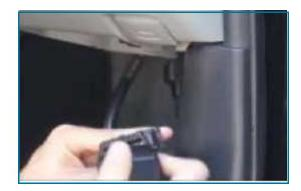
5. Cable tie the OBDII tracker into a secure position under the dashboard with the correct side facing upwards.
